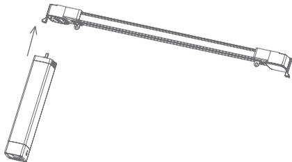
Step 2: Rotate motor and circlip reset automatically
